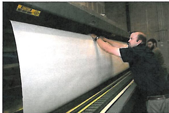
FAST SIGNS OWNER Jerry Hoyler loads his massive HP sign printer Aug. 13 in Goodyear. The printer can print signs in full color as large as 20 feet wide. Those pieces can then be welded, or bonded, together to create even larger signs.
